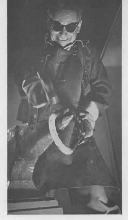
MOST MODERN of welding shops, such as Sandia's, must occasionally use ancient techniques of metalworking for a particular job. Fred Buttrey hand-shapes a part using hammer and anvil. Piece was torch heated.
